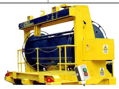
Self-Powered Live Cable Reel developed to feed electricity to the big mining shovels when travel from one position to a new one.
