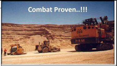
Picture shown one of three LCR-1200's being towed by a wheel dozer at the same speed of a 2800 MK2 P&H shovel at the Mina Sur minesite, Codelco Chile.
