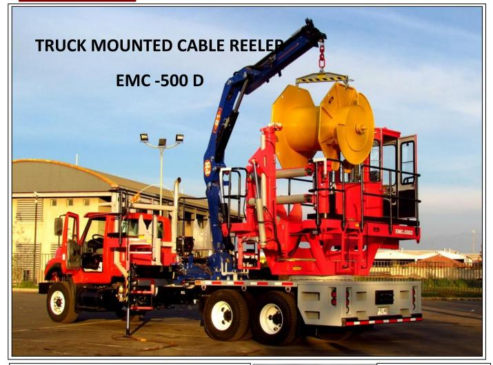
The **Truck Mounted Cable Reeler EMC-500D** is the latest design and meets all requirements for the mining electric cable handling. This new version is easier and safer for the operation, full remote control for crane and reeler, isolated cab and better visibility than the previous models. Its features are:
