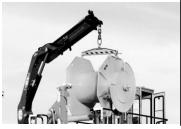
Two drums mounted allow the cable reeler work with 3000 Ft of electric cable at a time.
